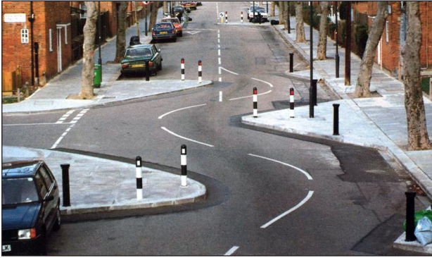
Speed Tables, Chicanes, and Pinch Points (County Surveyors Office 1994)
