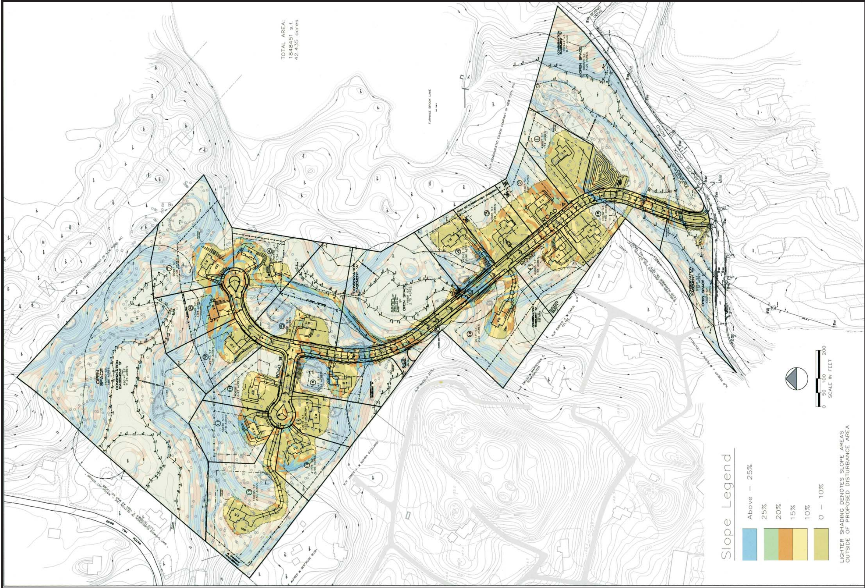
Figure 1-2: Proposed Plan / Slope Disturbance Furnace Dock Town of Cortlandt, Westchester County, New York Source: Ralph Mastromonaco, P.E., P.C. 6/27/05 Scale: Graphic
