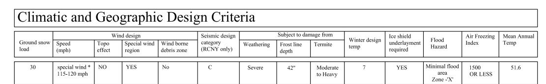
115 mph to 120 mph. The special wind region should serve as a warning to design professionals in evaluating wind loading conditions. Wind speeds higher than the derived values taken from section 1609 of the IBC and figure R301.2(4)A of the IRC are likely to occur and should be considered in the design
