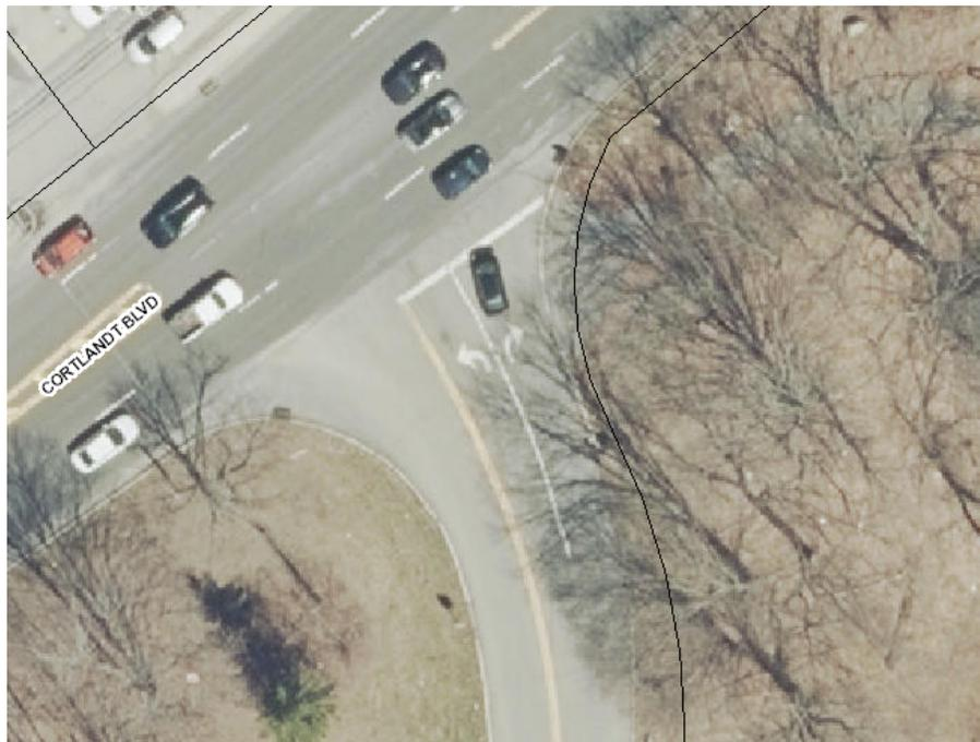
Regarding adding a left-turn lane on eastbound Route 6, there is an insufficient distance between the existing westbound Parkway off Ramp and the Bear Mountain Parkway overpass to construct a left-turn lane that would comply with the minimum NYSDOT standards (see below).
