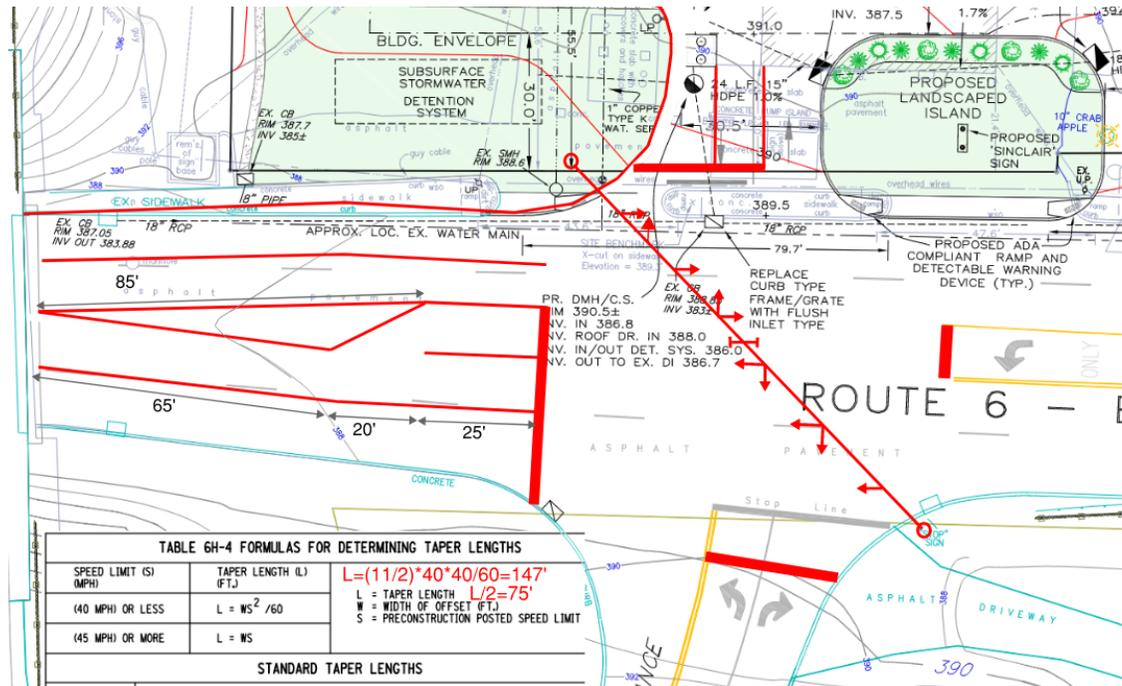
While it would be desirable to provide an eastbound left-turn lane, for signalized intersections, the AASHTO Policy on Geometric Design of Highways and Streets recommends (on page 9-109) that "left-turn lanes should be considered where left-turn volumes exceed 100 veh/h". The maximum projected left-turn volume on the eastbound left-turn movement is just 65 veh/h.
